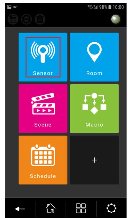
In the sensor menu click on the “Gear Icon” in the top left corner and select “Clear all device”. After this a new window will open check mark “Confirm To Reset” and click “ Clear All” All devices will now be removed. Logout of the APP and Login again the Device will not be shown. Scenes and Macro’s can be deleted one by one.
